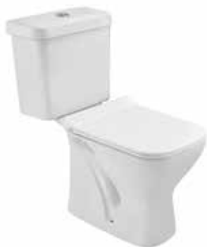
AIS-WHT-101751S220SPPSMZ Bowl With Cistern For Coupled WC With PP Soft Close Slim Seat Cover, Hinges, Dual Flush Cistern Fitting, Fixing Accessories and Accessories Set, Size: 395x680x775 mm, S Trap- 220 mm
